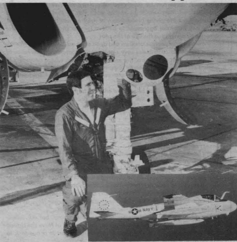
DEADLY TURRET — Lcdr. Pete Dabbieri, the A-6 Software Support Activity's project pilot, checks out the A-6E Intruder's Target Recognition and Attack Multisensor (TRAM). The turret contains equipment that can detect and identify a target in total darkness. —Photo by Ron Allen
