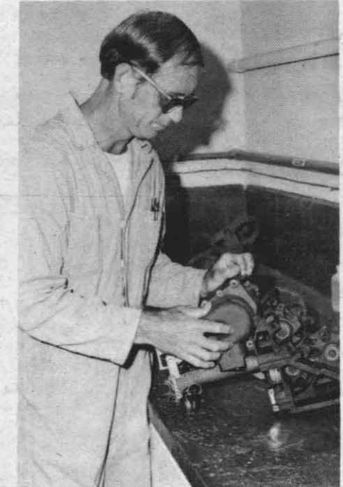
JAMMED MECHANISM — EMCM Jerry Banister prepares to remove eight live cartridges jammed into an M61 machinegun breach mechanism. The work is being performed in the Explosive Ordnance Disposal Detachment's breakdown building.
