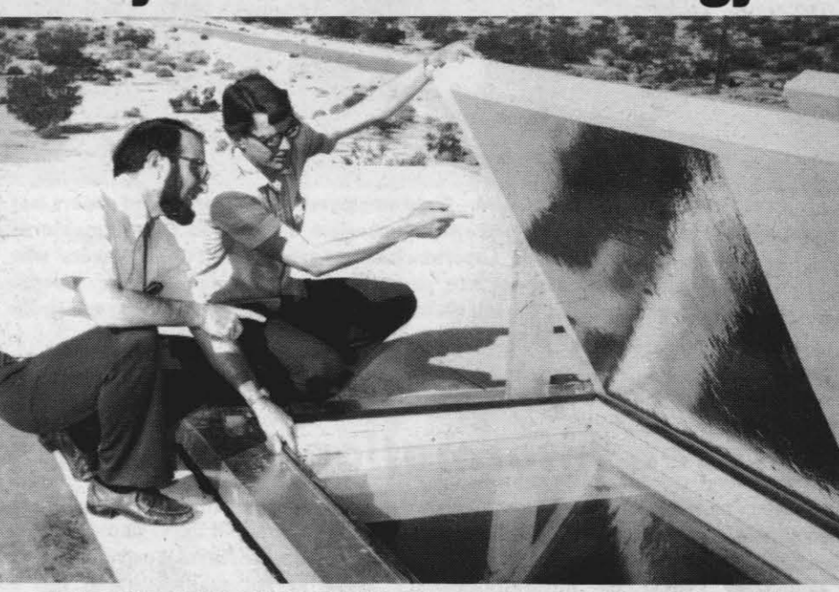
LIGHT AND HEAT REFLECTORS —Richard Fulmer (left) and David Wirtz inspect the light louvers on the Center's experimental Low Energy Structure test cell. Fulmer is the head of NWC's Energy Program Office, while Wirtz heads the LES project for the Ordnance Systems Department's Advance Technology Division. The reflecting surface on the louvers direct sunlight and solar heat into the building during winter. The louvers seal at night and are made of polyurethane foam covered with glass cloth and resin. In the winter the louvers face the south for greater heat and light; in the summer they face the north. —Photo by Alan Fry
