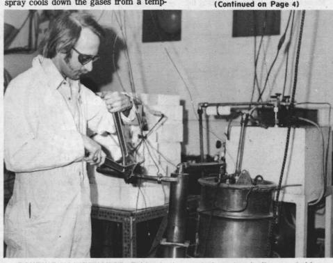
ROUTINE MAINTENANCE—Tubing in the pyrolysis system is disconnected by Jim Diebold and cleaned out after a test run to insure continued smooth operation.
