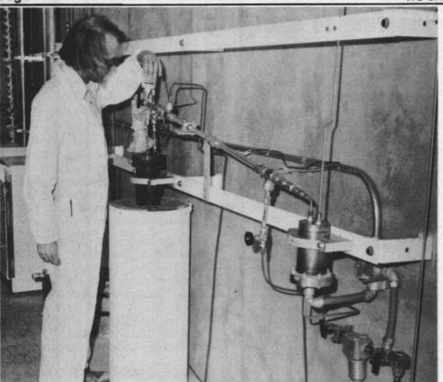
CHECKING FOR LEAKS—Before starting another test run, Jim Diebold checks the high pressure polymerization reactor for any leaks. Gas pressure in the reactor during a test run is 750 pounds per square inch.
