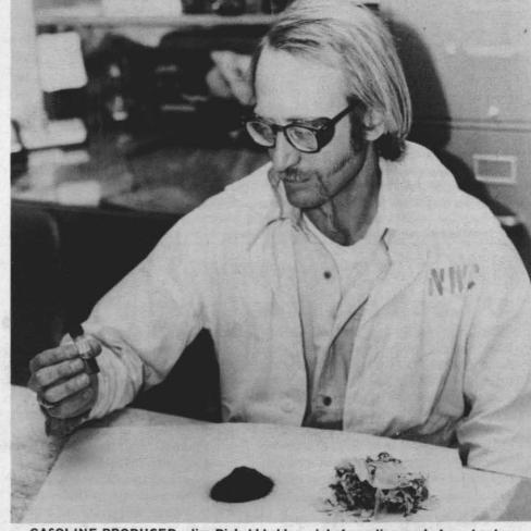
GASOLINE PRODUCED—Jim Diebold holds a vial of gasoline made from trash which is the product of a bench-scale pyrolysis, gas purification, and polymerization system developed here. The solid waste feed stock (the fine powder seen in center) started out originally as scraps of paper, plastic, feathers and other cellulosic organic waste material (at right). —Photos by Ron Allen
