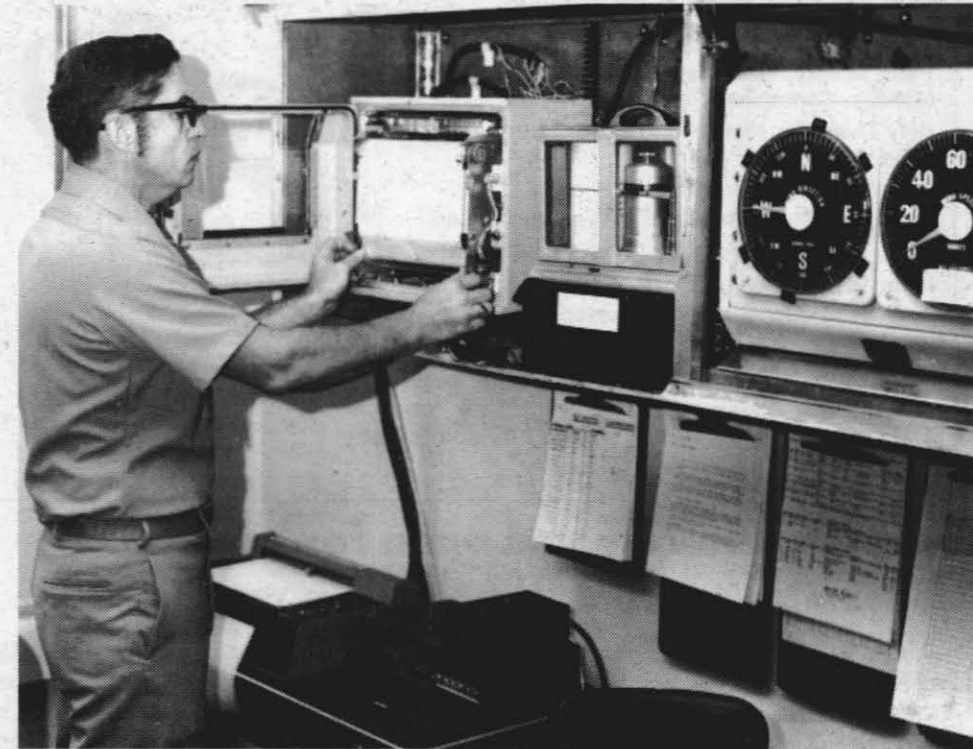
CHECKING THE WIND —Chief Aerographer's Mate Chelmer E. Finger adjusts a wind recording instrument at the Naval Weather Service Environmental Detachment office at China Lake. Winds generated by Sierra waves often exceed 80 knots here. —Photo by Ron Allen
