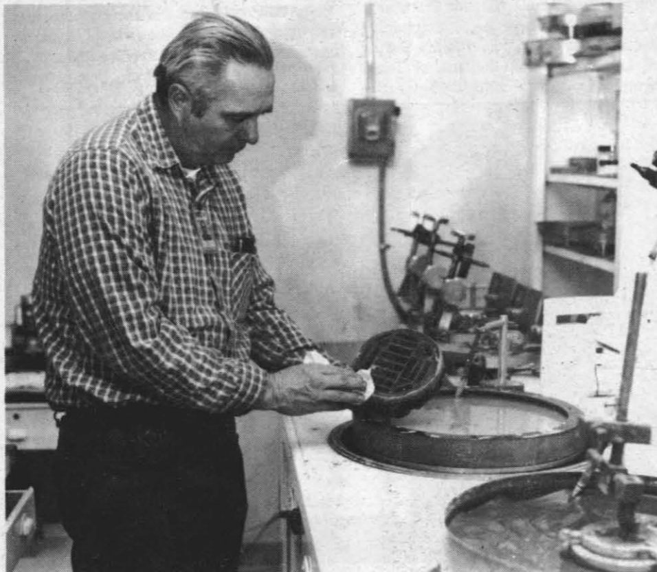
CHECKING THE WORK — Joe Shaffer checks prisms imbedded in a plaster compound to hold them in place for surface polishing in the bowl feed polisher seen above. The bowl feed polishing devices run 24 hours a day to produce the finished surface sought on lenses, prisms, and mirrors. —Photo by Ron Allen
