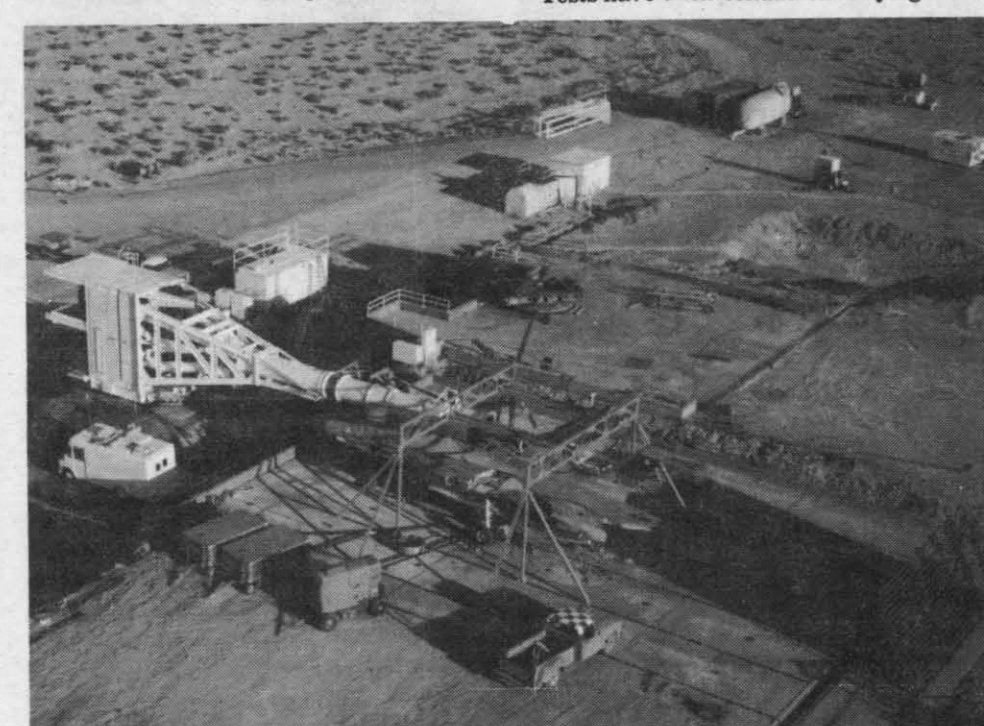
AERIAL VIEW OF TEST FACILITY — As this photo of the Aircraft Survivability Program test site was shot by Sam Wyatt, the horizontal, tower-like structure (called the Dash airflow facility) was being used to simulate airflow over the wings of an F-14 Tomcat aircraft during a test conducted to evaluate the aircraft's fire extinguishing system.
