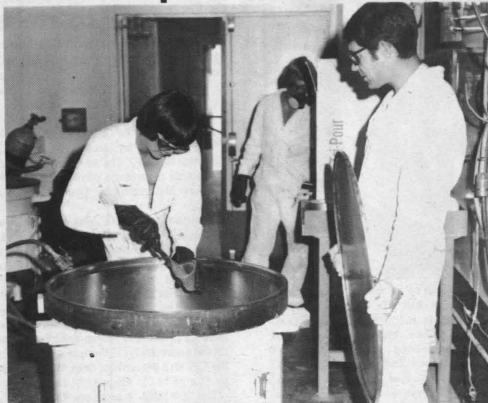
PREPARING FOR VISCOSITY TEST — After being mixed, a sample of an inert solid propellant is being removed by Michael Knight (at left), an explosives worker in the Explosive and Propellants Processing Branch, in preparation for running a viscosity test. The lid of the 25 gallon mixer has been removed and is being held by Howard Gerrish, a chemical engineer. In the background (wearing a mask over his face) is Robert Tremonte, an explosives operator.
