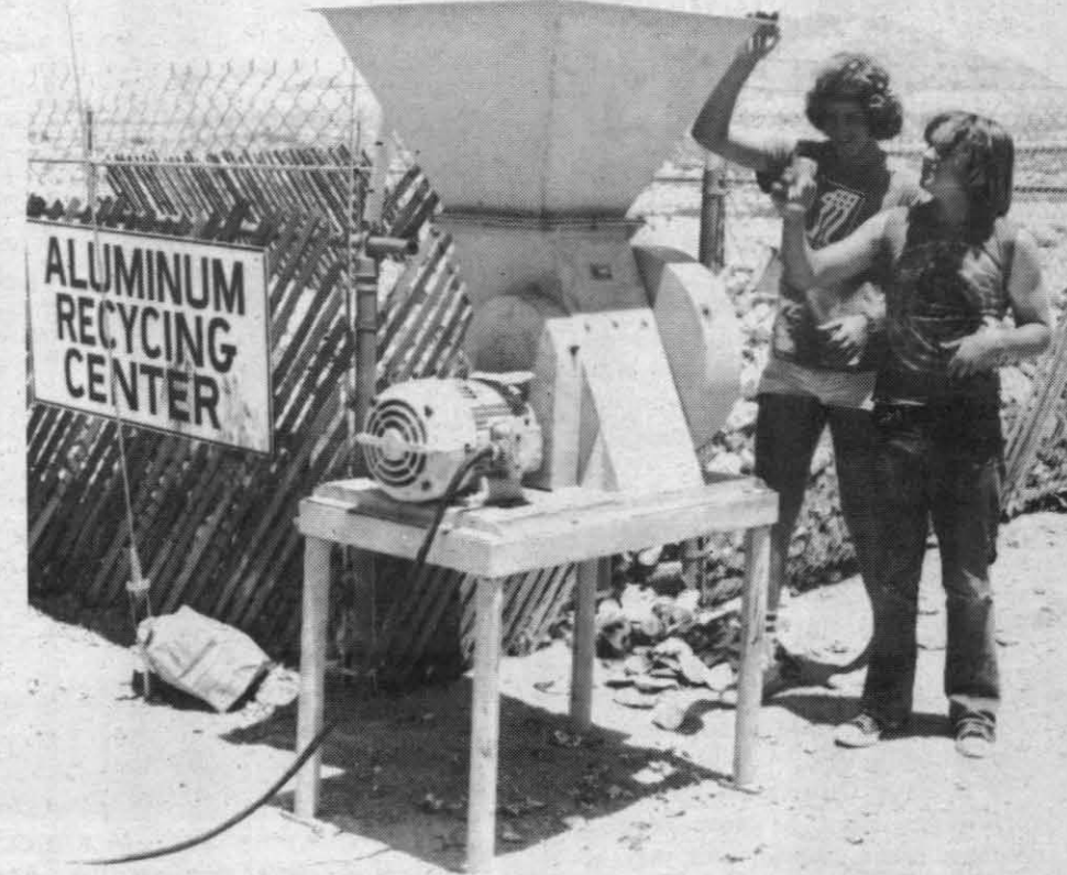
BUSINESS IS PICKING UP — A machine for shredding aluminum cans, which has been installed at the community recycling center, is shown being operated by Robert Pooler and Craig Davis, two of the center's volunteer workers. Also being collected at the recycling center, which is being operated under the direction of an Employee Services Board committee, are glass bottles and old newspapers.
