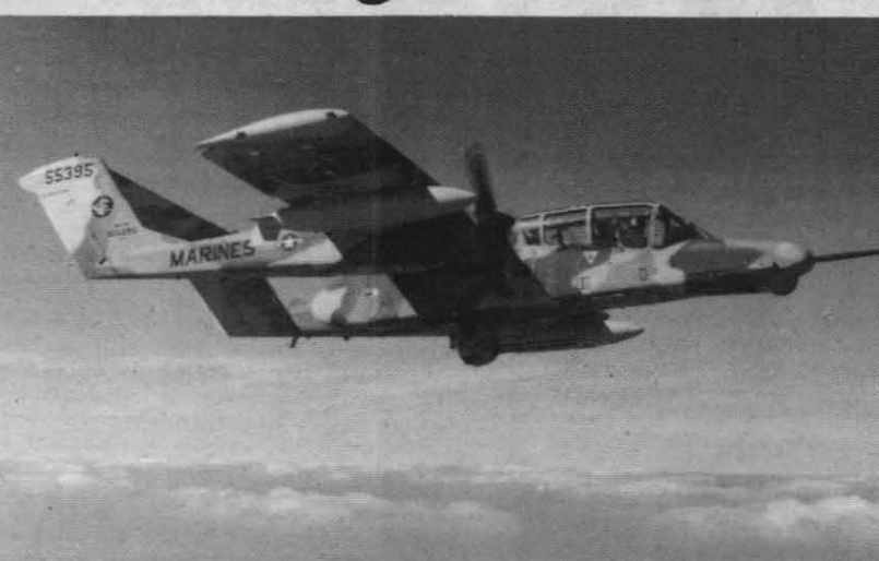
FLYING HIGH — This OV-10D Night Observation Surveillance aircraft is now undergoing propulsion flight testing at the Columbus Aircraft Division of the Rockwell International Corp. Its length is 41 ft., 7 in., the wingspan is 40 ft., and it can carry a crew of two (pilot and observer).
