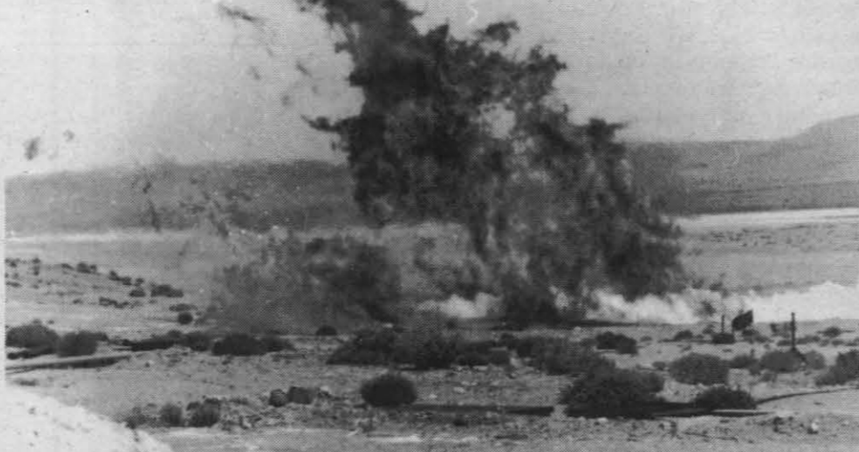
TESTING PROGRAM CONTINUED — After a six-month wait for the right wind conditions, another in the series of tests under the Vapor Cloud Explosion Study was conducted here recently at test area CT-6 under the supervision of the program manager, Dr. Doug Lind, who works in the Propulsion Development Department's Explosives Technology Branch. For the test, 1,500 gals. of liquefied natural gas (LNG) at a temperature of minus 160 degrees C. was spilled on a pond of water. Boiling on the surface of the pond, the LNG evaporated very rapidly and formed vapor, which in turn condensed water vapor out of the air—visible as a white cloud of fog in the above photo. The flame is from the clean-burning LNG. Data from the test, which took about two minutes to complete, is still being analyzed; already, however, it has been learned that the vapor did not burn back significantly to the place where the spill originated, but only where it had blown downwind of the spill. Further tests are planned under different wind conditions and with variations in the time of ignition. The study is being sponsored by the U.S. Coast Guard. —Photo by Randy Eady
