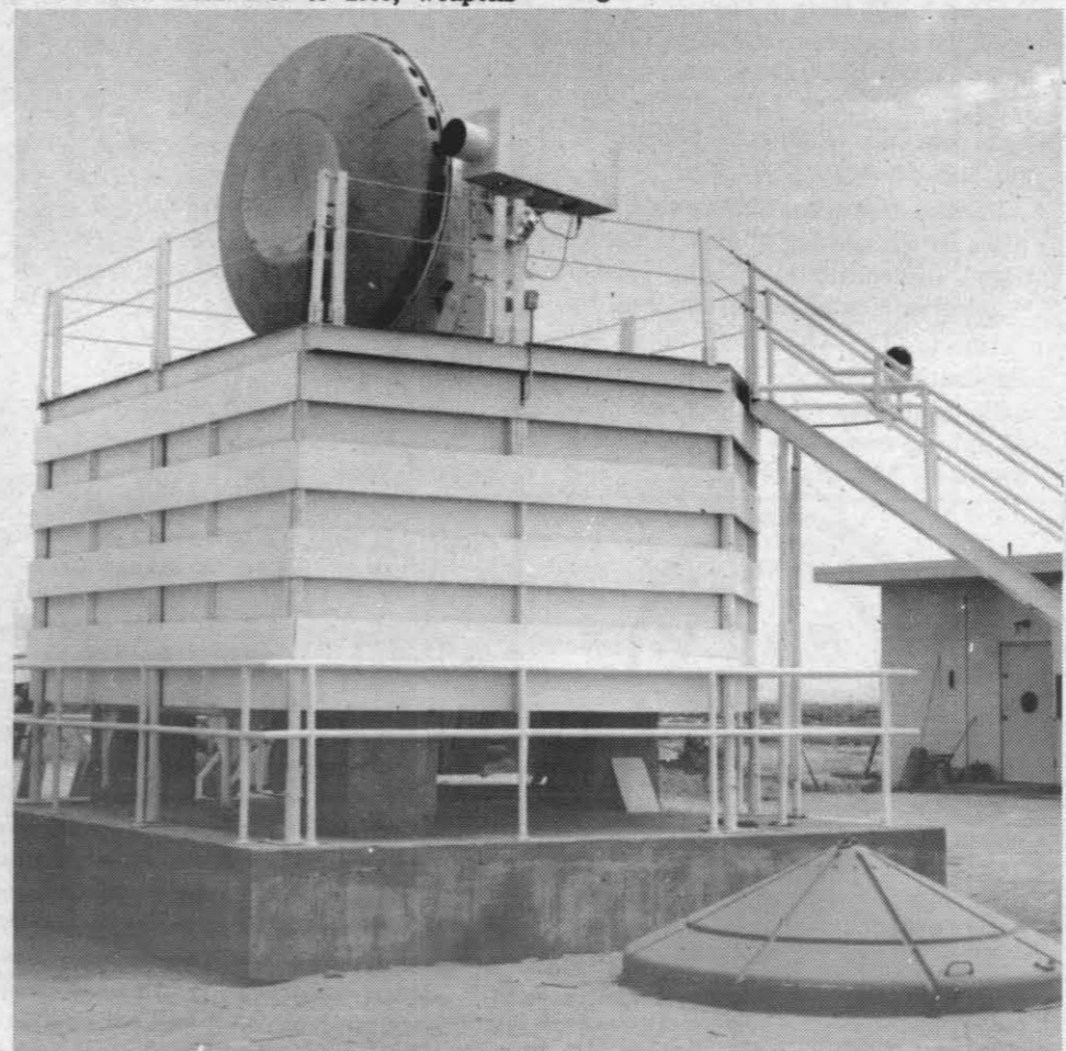
SPECIAL FEATURES OF ON-AXIS RADAR SYSTEM — At the north G-1 range tower 9 Nike-Hercules radar site can be seen a star calibration camera and 120-in. lens mounted on the on-axis configured radar. By the use of star-field calibrations and prediction techniques in conjunction with a computer, it is possible to correct (in-real-time) systems errors and accurately track range targets.
