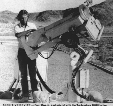
SENSITIVE DEVICE — Paul Owens, a physicist with the Technology Utilitization Office of the Propulsion Development Department, checks the alignment of the mirrors on the circumsolar telescope which is located on the roof of the Research Department's Earth and Planetary Sciences Building. Developed by the Lawrence Berkeley Laboratory, the telescope has a rainflap which may be seen at the upper -Photo by Sam Wyatt that have been emplaced at various
