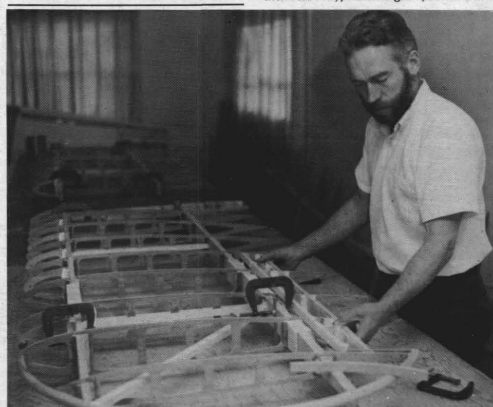
PROJECT HALF COMPLETED — Bill Hickie is shown fitting the ailerons to the lower wings of his half-built Pitts Special biplane. This aircraft has special characteristics that make it especially suitable for the aerobatics maneuvers which its owner enjoys performing in the skies around Inyokern.
