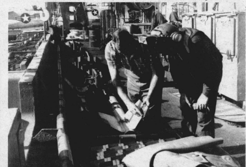
HELPFUL DEMONSTRATION —Procedures for checking the roller on cager assembly on the Sidewinder missile are demonstrated by Ken Ayers to a member of the USS Roosevelt's air-launched missiles crew. Frequent visits by Code 366 personnel to the Fleet help keep important communication channels open for rapid response to Fleet engineering problems.
