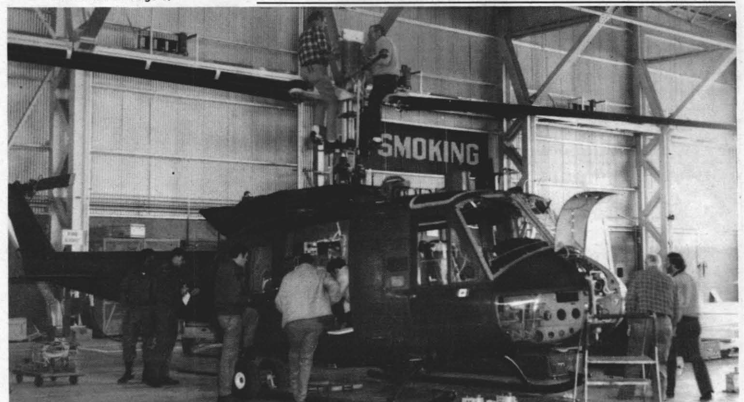
HELICOPTER DEICING SYSTEM TESTED — Two contractor personnel from Lockheed-California (Bob Lennard, at left, and Ralph Metcalf) are shown closing up the instrumentation package atop the main rotor mast of a UH1H "Huey" helicopter in preparation for conducting tests of the "chopper's" deicing system. Other members of the test team involved in this work are (l.-r.) Army S/ Sgt. Vern Taylor, helicopter crew chief; Navy Lt. Mike Hill and Army Capt. Eugene Mace, test pilots, and Steve Kiser (back to camera), an instrumentation engineer from Lockheed. At far right are two more contractor employees — Dick Hillman, an instrumentation technician, and Len Macy, flight test engineer. —Photo by Sam Wyatt
