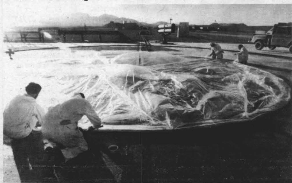
MAKING READY — A plastic film hemisphere with a 10 meter radius is fastened to a wooden ring on a concrete firing pad in preparation for inflating it with a fuel-air mixture. The resultant "cloud" was later ignited by electric spark as part of the second phase of the "vapor cloud explosion study."
