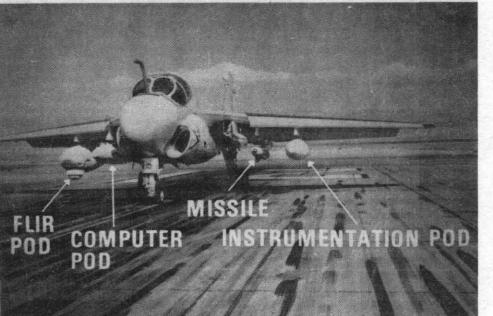
READY FOR FLIGHT TEST - Headed for Airport Lake range, this Navy A-6 Intruder is about to take off for a free flight test of the Night Attack / Maverick missile. This night attack version of the missile makes use of a forward-looking infrared (FLIR) sensor for target acquisition. Both a computer pod containing the boresight / aimpoint correlator pod and an instrumentation pod used to record performance data are attached to the aircraft for test purposes.
