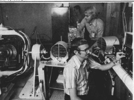
SEEKER PERFORMANCE CHECKED IN LAB - Don Watke (in foreground) is shown with Heinz Roesser and Michael Pullen (standing in background) as they make use of a three-axis flight simulation table to check out the operation of the Maverick missile's night attack seeker. Work such as this was a prelude to the successful flight tests of the missile during which direct hits were scored on the
