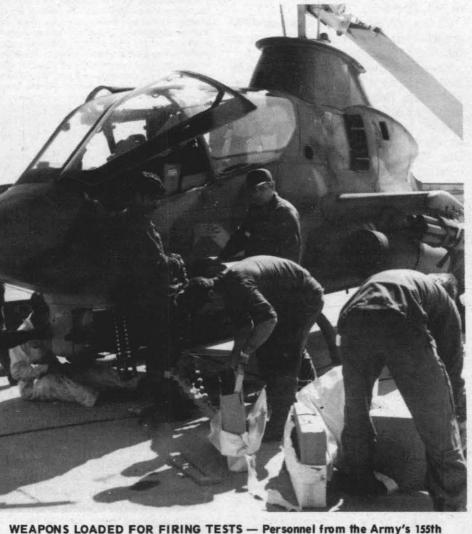
Aviation Company are shown loading 40mm guns in preparation for extremely low level firing runs by AH1G Cobra helicopters at the Airport Lake range. In addition to the 40mm guns, the helicopter pilots also fired 2.75 in. folding fin aerial rockets and 7.62mm machine guns.
