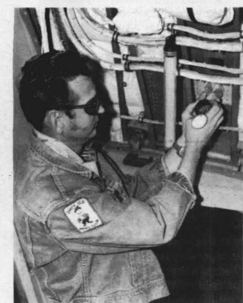
NEW EQUIPMENT — Modifications to the National Research Foundation's LC-130R Hercules have included a dewpoint hydrometer which Dan Blackburn, an aircraft metalsmith, is shown installing. —Photo by Ron Allen
