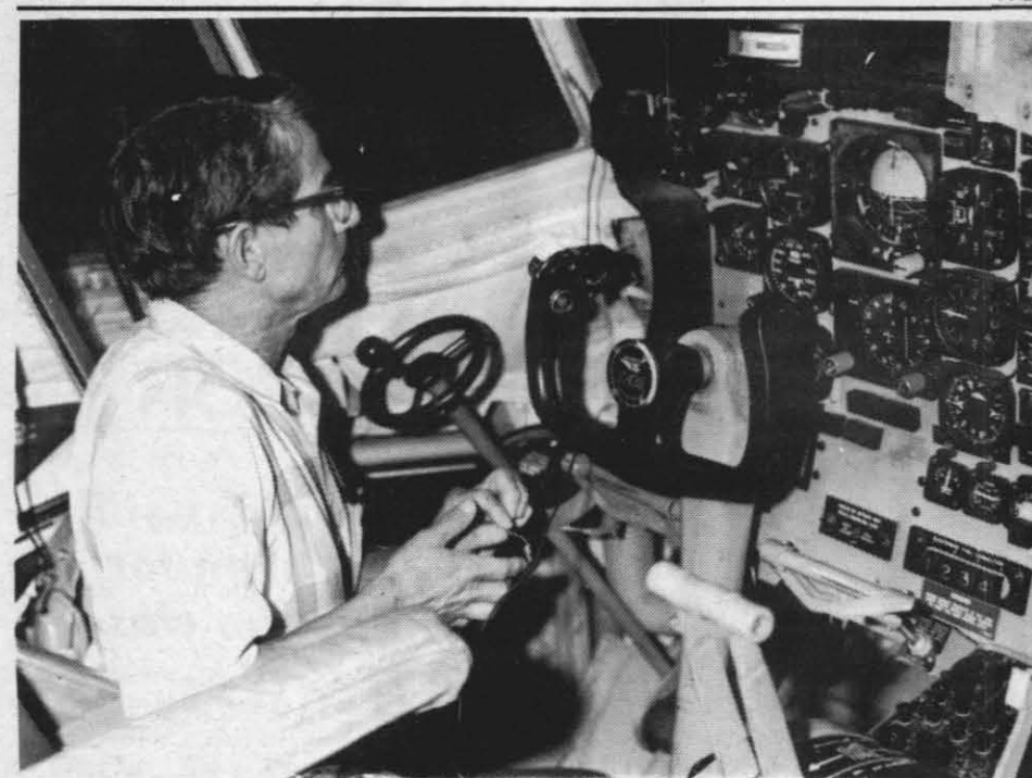
INSTRUMENT PANEL INSPECTED — Richard C. Chatterton, design engineer in Code 3712, checks out the instrument panel of the LC-130R Hercules following installation of the NWC-developed data acquisition system in the huge National Science Foundation aircraft that is used for research in the Antarctic.
