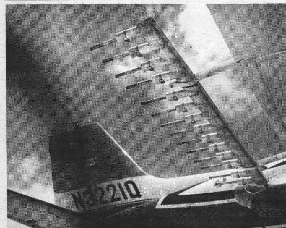
CLOUD SEEDING AIRCRAFT ALOFT — There are 14 Fuze E type dispensers used for cloud seeding mounted on the wing of this Cessna 401 aircraft. Materials released from dispensers such as this can be used for seeding squall lines or clearing away super-cooled fog. Equipped in the above fashion, this aircraft was used for successful weather modification work in Florida, Texas and other parts of the U. S., as well as in Panama and over the Barbados Islands in the British West Indies.
