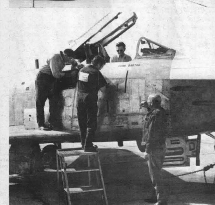
QF-86H DRONE PRODUCTION PROGRAM COMPLETED — In slightly more than two years' time, the production phase of the program to convert the airframes from Air Force F-86H Sabrejets into 29 remotely controlled subsonic target drones was completed. This was no small task, as can be seen by the photo at top left which shows what condition some of the aircraft were in before this work began. The conversion program involved NWC civilian and military personnel, aided by contractor employees. In photos typical of the work that took place, George Mullett, associate head of the NAF Targets Department, may be seen in the picture at top right adjusting an item of ground test equipment that was produced for this program by employees of Code 3925. In
