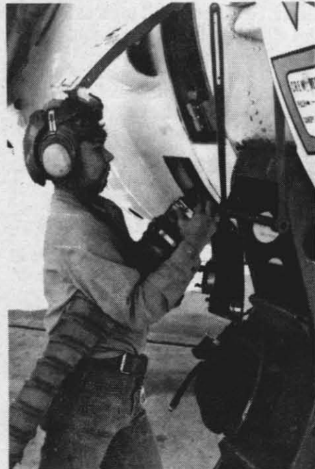
ENGINE STARTER — ADJ3 John Dempsey connects an air hose, called "the huffer," in preparation for starting the engine of a Grumman EA-6B Prowler. The air pressure turns the turbo jet's turbines until they reach a high speed high enough to start the aircraft's power plant.
