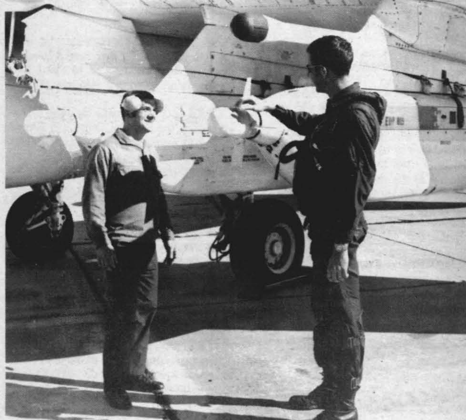
THIS DOES THE TRICK — Lt. Bernie Hedger, of VAQ 136, checks over the jammer pod that plays hob with the effectiveness of ground or shipborne radar. Lt. Hedger has his hand on the propeller blade of the jammer pod's ram air turbine. Looking on at left is AHH1 Larry Gregory.
