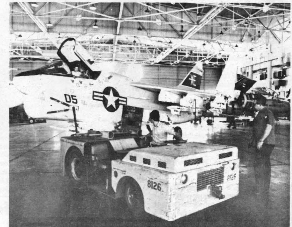
SN K. A. LOCKWOOD is preparing to hook up to the A-7 Corsair II in the background prior to towing the aircraft on the line for a "launch." In the cockpit is AA Julio Huete, who will "ride the brakes." Ginter watches the operation.
