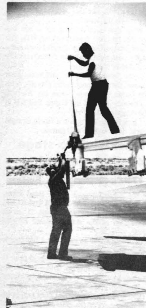
AA MAJOR WILLIS and Ginter are placing wing locks on an aircraft. "The wind knocks the wings down if this isn't done," he noted.
