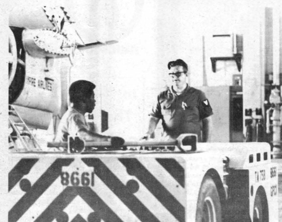
THE LINE supervisor is always present when aircraft are being moved into Hangar 1. Here, Ginter directs AA Major Willis, who is driving a "tug," Navy slang for an aircraft tow tractor.
