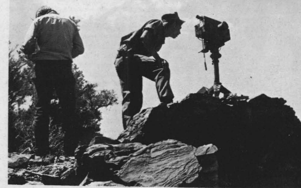
JOINT TEST HELD —An unidentified Marine peeps through a ground-based laser designator while a civilian employee of the Naval Weapons Center records data passed on to him by the military man. The photo was taken during a recent three-week joint operational test of laser-guided weapons in close-air support held at NWC. The laser designator above illuminates the target with a laser beam. The reflected beam was then detected by a seeker system on A4M Skyhawks flown by pilots from VMA 214 at El Toro. This provides guidance to both the aircraft and the weapon for the drop.
