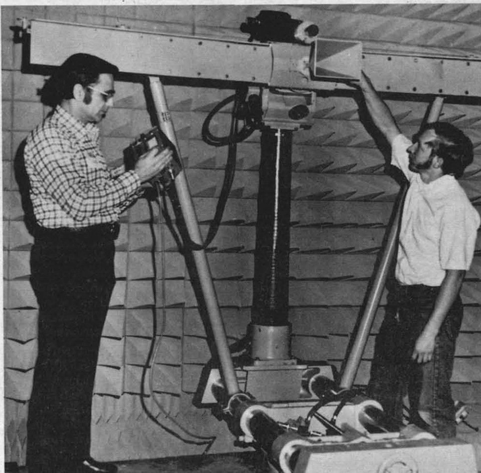
HAVE TECHNICIAN, WILL TRAVEL — Charles Gibson (r.), a model-maker at the Salt Wells Machine Shop, is shown assisting Dave Scoles, a mechanical engineer with the Engineering Department's Control Design Branch, in setting up a moving target simulator for use in making tests for an approved radar missile target seeker for Sparrow AIM-7F. The tests were conducted in the anechoic chamber. Gibson was loaned to Scoles to help build the apparatus and assisted with the drafting and design of the fixture. Bill Danley, who heads the machine shop at Salt Wells, has other men available for this purpose, plus all of the machine tools, drafting tables, etc., needed to complete a task. Scoles and Gibson began building this special apparatus in January. The horn at the top moves along the T-bar rail at various speeds, ranging from 1 in. per second to a very high rate. Scoles holds the control box that operates what he calls a "soap box derby steering system" for this special piece of equipment. He came to China Lake in February 1971 from Corona where he had been employed since June 1956. —Photo by Ron Allen
