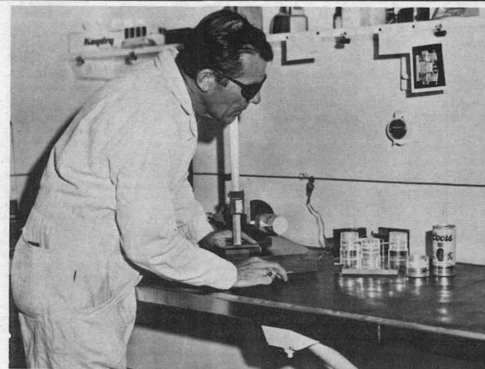
GETTING READY FOR TEST — Ed Brehmer, a mechanical engineering technician, is shown making final adjustments on a test unit designed by Gordon Greene, a physicist in Code 4541, just prior to moving the experiment into a firing bay and initiating the explosive. In this particular test, discarded aluminum beer cans are being used as the container for holding either liquid or putty-like explosive materials. —Photo by Maurice Dias
