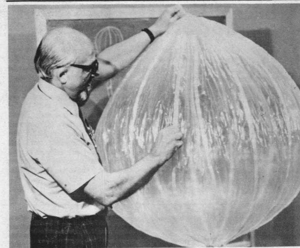
MODEL OF PROJECT da VINCI BALLOON —Heat-sealed, reinforced seams of the 70-ft. tall balloon that will carry scientific instruments and four researchers on an experimental flight to study elements of the lower atmosphere are shown on this model of the helium-filled balloon held by Karl Stefan, the project's balloon system engineer. Project Da Vinci is supported by the National Geographic Society, the Atomic Energy Commission, and the U.S. Army.
