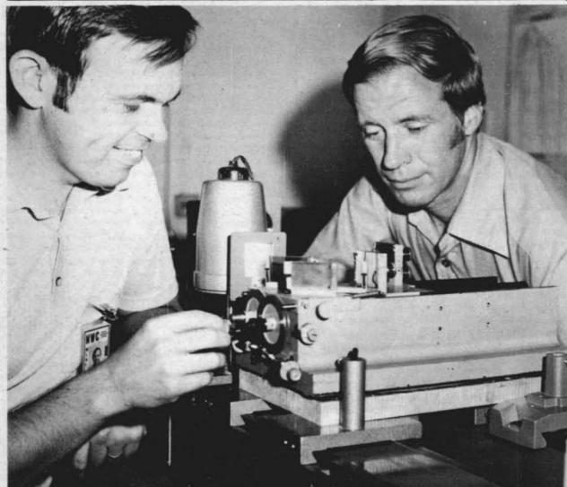
OLD INSTRUMENT USEFUL TODAY — Keith L. Gardner (at left) and Donald W. Peterson, two physicists in the Weapons Development Department, have found the Michelson parallel path interferometer highly useful in their current work on an advanced electro-optical system. This instrument, similar to one used by Dr. A. A. Michelson in 1892, was borrowed from the Michelson Museum on the Center. Gardner and Peterson are shown adjusting the path length on the interferometer.
