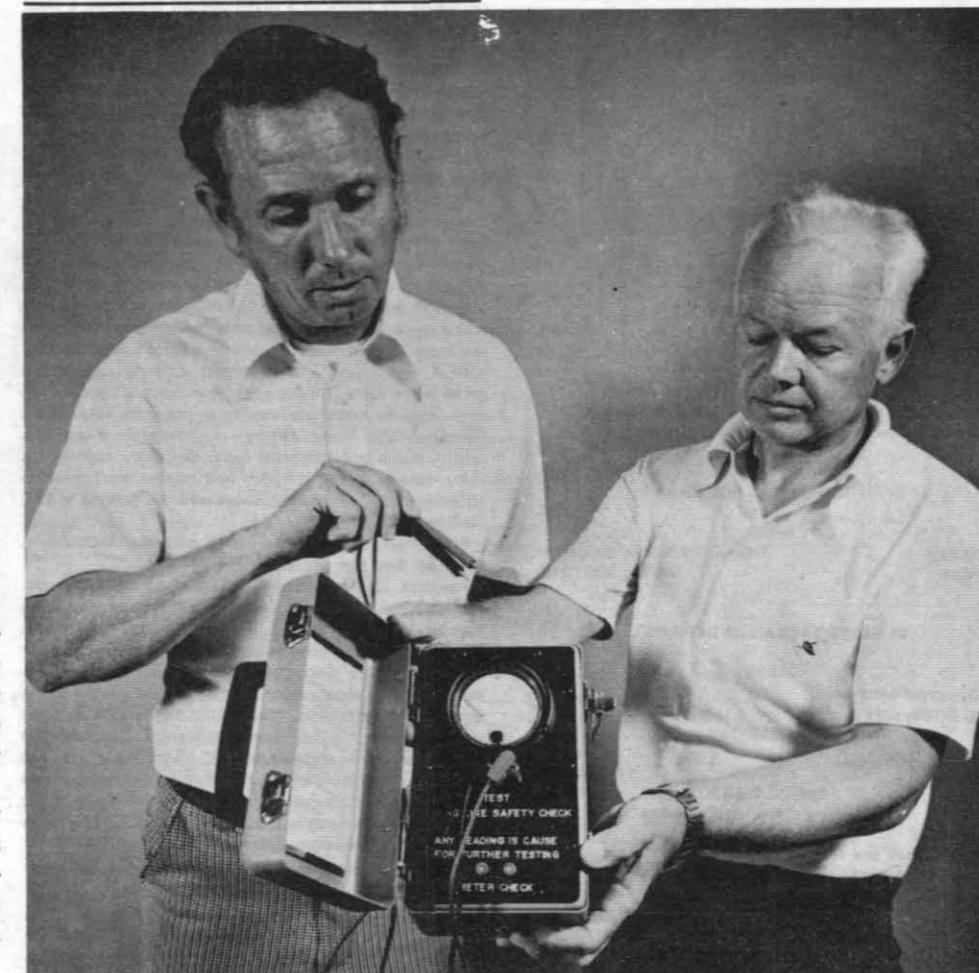
NEW MEASURE OF SAFETY — Roy Johanboeke (l.), head of the Ballistics Test Branch in the Propulsion Development Department's Quality Assurance Division, and Robert Meade, an employee of that branch, display a no-voltage meter, developed recently by Meade. This simple test set can be used to determine whether there is electric power, either AC or DC, running through a firing line prior to its hook up to a charge. —Photo by PH2 D. W. Yeatts
