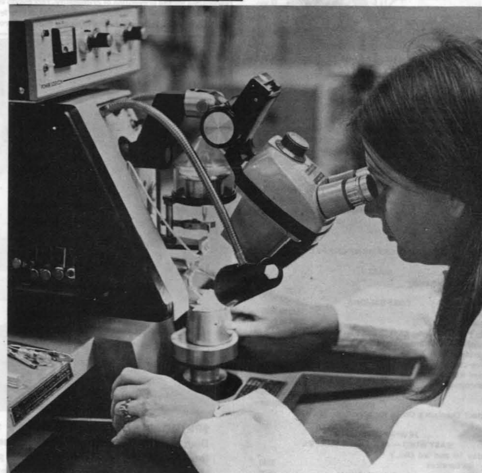
THIS IS AN ultrasonic gold wire bonding machine that is used by technicians of the Microelectronics Branch to electrically connect various components to the conductor runs. The machine uses gold wire that is .001 in. (1 millimeter, in diameter). The operator in this photo is "Sam" Shaffer, an electronics mechanic.
