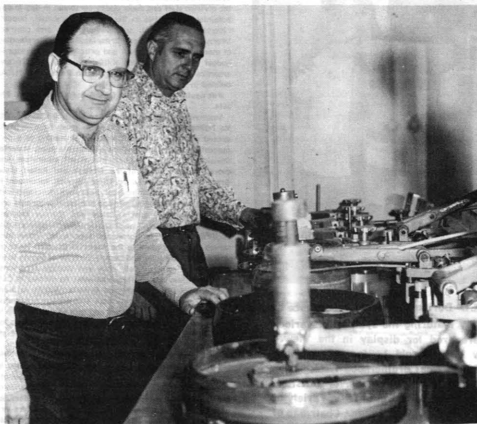
POLISHING SPINDLES —Don Bevis (left) and Joe Shaffer display some of the polishing spindles they use at the NWC Optics Shop to turn out optical surfaces that are typically three to four times as smooth as the surfaces produced by commercial techniques. With 4 grinders and 12 polishing spindles, the Optics Shop is now better equipped than ever before in its history.
