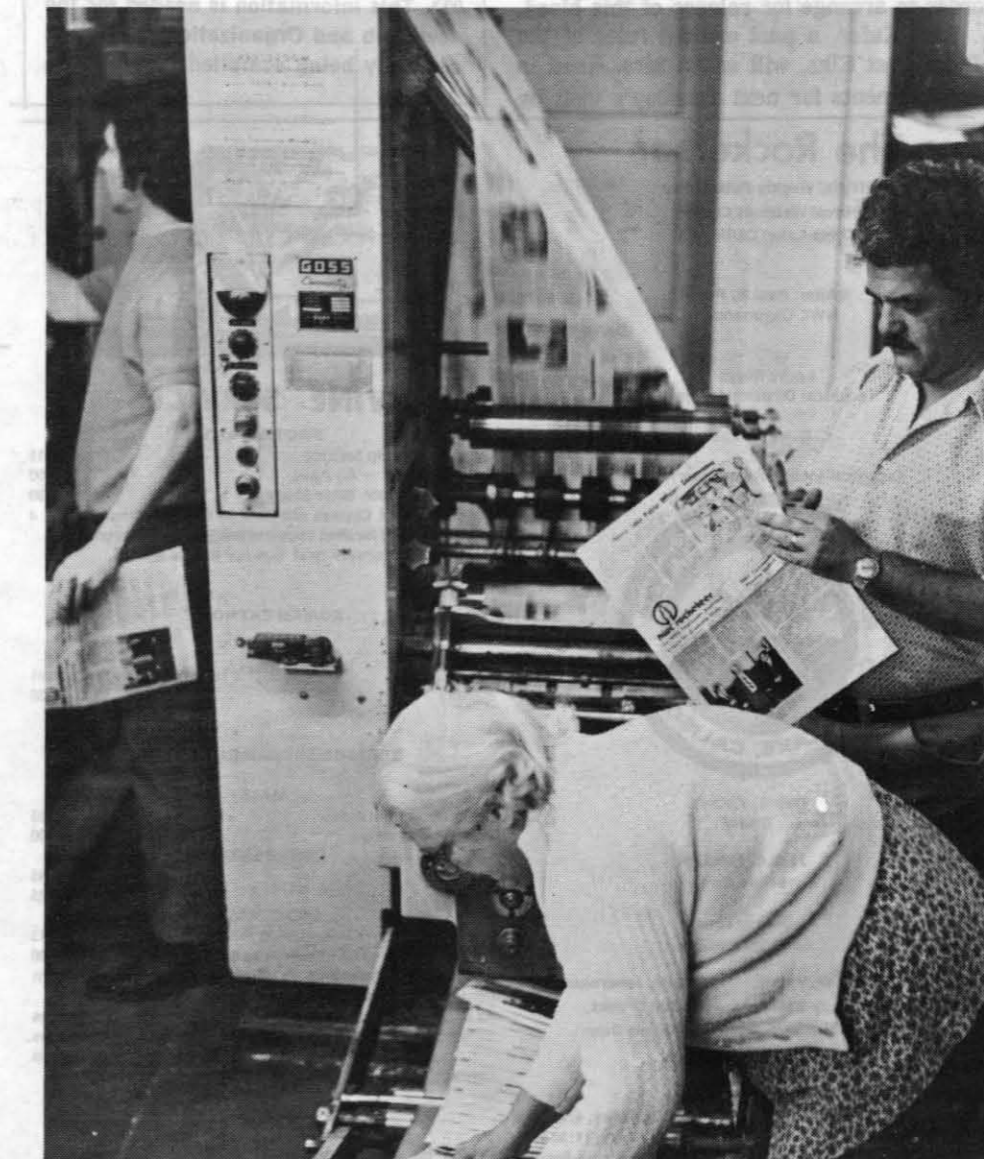
HIGH SPEED PRESS — Jack Lindsey, ROCKETEER associate editor, checks one of the early copies of the newspaper during the press run on Friday mornings. The Goss Community press in use at The Daily Independent, where The ROCKETEER is printed, runs at 12,000 copies per hour at the top of the scale. At left, Dwight Quick, the pressman, is seen adjusting the flow of water to the press, while Mary Post can be seen gathering the papers for tying and bundling.
