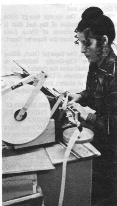
TYPESETTERS — Sharon Robinson (above) is seen typing ROCKETEER articles on a tape puncher. The tape is then run through a computer which justifies the type to the pica size desired. Below, Penny Chase is typing correction lines following the Friday morning reading of the pages by staff members.
