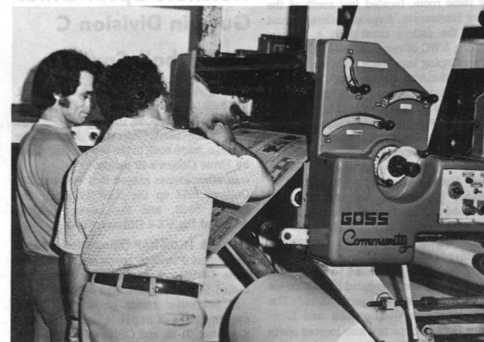
FINAL PAGE CHECK — Jack Lindsey, associate editor, reviews a "plate," from which the newspaper is printed by the offset process, prior to the press run. Dwight Quick also helps in this procedure.
