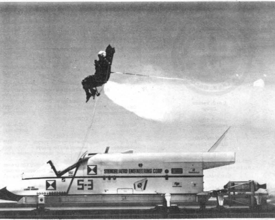
A SHOOTING STAR — An anthropomorphic dummy played a starring role during the test of the SIIIS-3 ejection seat at 435 knots in air speed, pictured here only milliseconds following ejection. Notice the canister is already popped open and the chute will open in 3 sec. following the separation of the seat and the aircraft.
