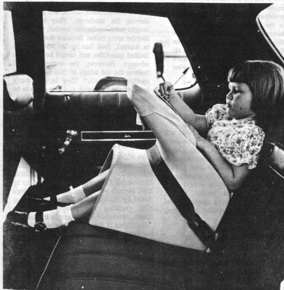
THE NO. 1 CHOICE — Lynda Specht, daughter of Mr. and Mrs. Kenneth Specht, demonstrated the No. 1 choice of safety experts in child restraint systems—the Ford Tot Guard. This particular seat not only holds a child in place in case of a sudden stop or collision, but soft polyethylene padding protects the face and bones of the tot.
