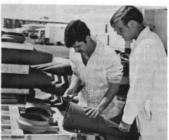
AO3 Charles Souza (left) and AO3 Rodney Patterson mount a tail fin on a bomb in the NAF Weapons Shop. All ordnance for aircraft is handled by this shop.
