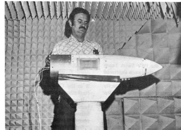
DICK WOOD is testing a fuze antenna on the Shrike guidance system.
