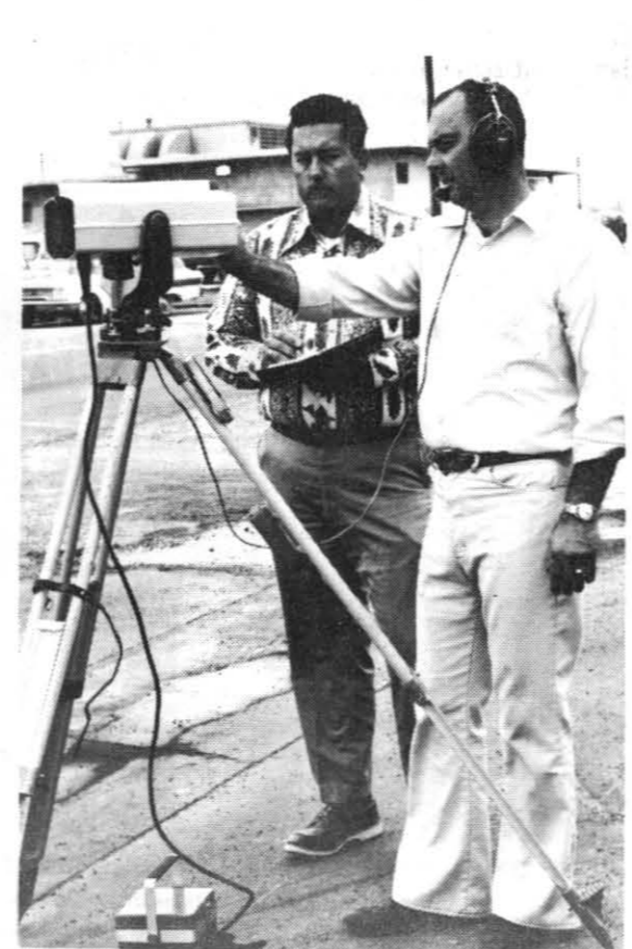
BILL KINGSLEY (left), a Co-op student from the New Mexico State University, at Las Cruces, adjusts the mirror lenses on his surveying gear, while in the right photo Jan Gieger (left), and Butch Lamson send an infra-red signal to Kingsley's apparatus. What they are using is a precision instrument that measures distances by infra-red signals to perform surveys. The equipment is accurate to 1/2 centimeter over a two-mile distance.
