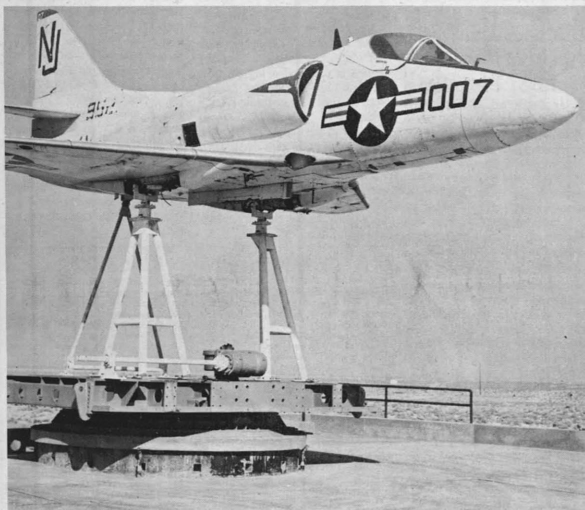
AN A-4 SKYHAWK aircraft, mounted on a test stand at the Aircraft Survivability Facility, awaits a test. With engines running, the aircraft will be impacted with small caliber ammunition at critical locations on the fuselage and wings to determine effect of impacts and extent of damage.
