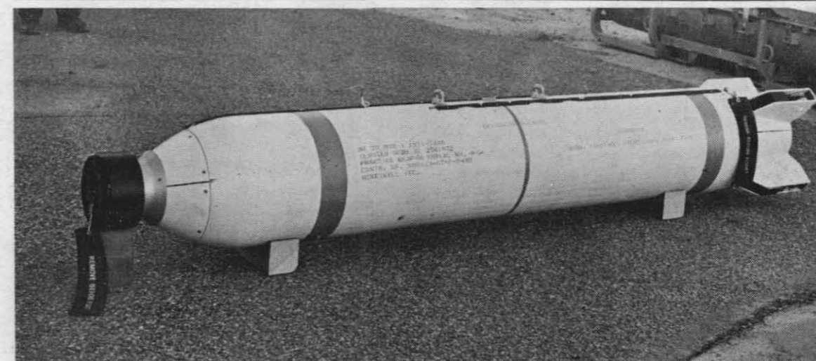
COMBAT PROVEN — Rockeye II, a weapon which has proven to be successful in combat in Southeast Asia, was designed and developed by scientists and engineers at the Naval Weapons Center. A 500-lb. unguided free-fall cluster weapon, it consists of a dispenser containing a cargo of 247 bomblets which pour out after Rockeye II has been released from an aircraft. Rockeye II can be used against such hard targets as tanks, armored vehicles and gun emplacements, or against such soft targets as trucks, parked aircraft and radar installations.
