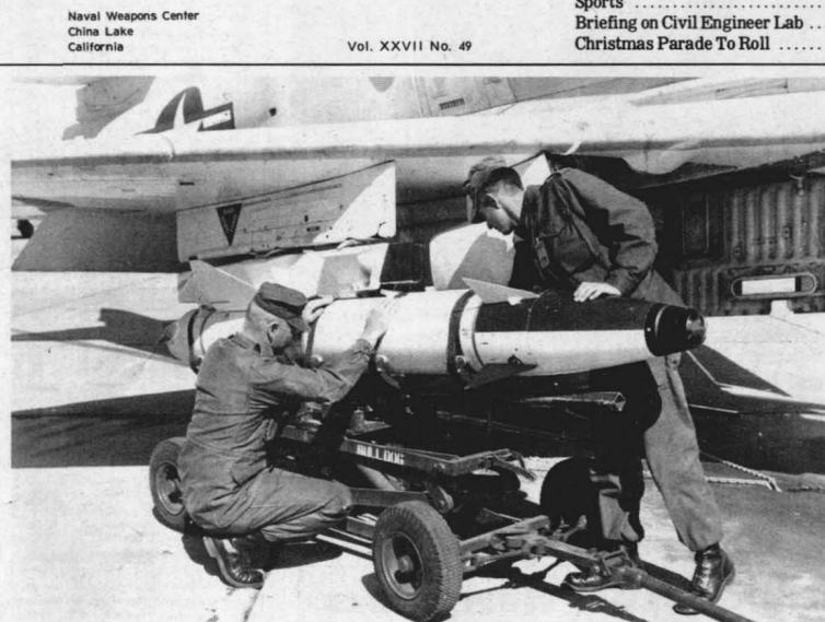
MARINES LOAD BULLDOG—Marines mount a Bulldog missile on an aircraft for flight testing on one of the ranges at the Naval Weapons Center. The Bulldog Weapon System, now in pilot production, was developed at NWC in response to the Marines' need for a close air support weapon. This laser-guided air launched missile provides first pass pinpoint accuracy in destroying surface targets.
