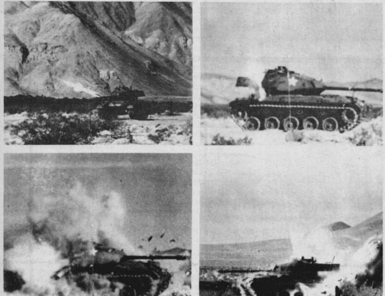
BULLDOG SCORES HIT—In this sequence of flight test photographs, Bulldog streaks toward its target, scores a direct hit, and demolishes it. This tank is one of a variety of targets used during flight testing of the weapon system.
