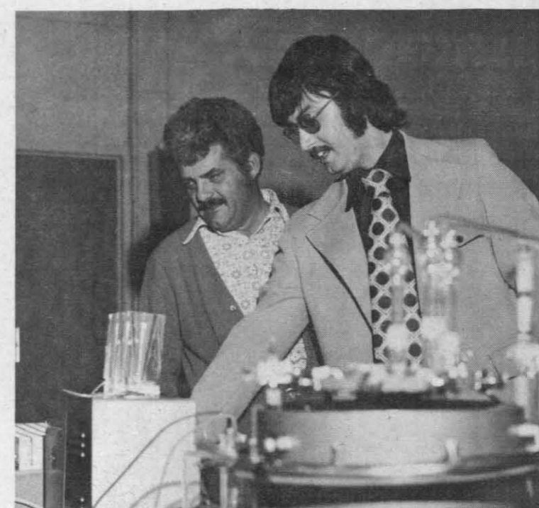
FRACTION COLLECTOR SHOWN —Mike Cammarata, a sales representative of Buchler Instruments Division, points out an interesting machine, known as the Fractomat 200, to the ROCKETEER reporter during a display of scientific apparatus equipment staged last Tuesday in the Community Center by VWR Scientific, a Los Angeles based firm. This fraction collector, as it is called, breaks down liquid mixtures and collects the individual components of the mixture into separate test tubes. It was one of many different types of apparatus on display during the six hour showing that was attended by many scientific and technical personnel of the Naval Weapons Center.
