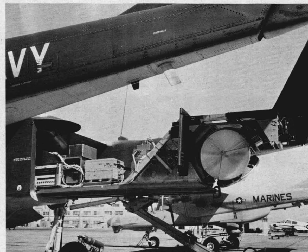
SPECIAL GEAR INSTALLED —Equipment that is used in a self contained position fixing and navigation system that has now been successfully flight tested by the Naval Weapons Center is shown as it was about to be installed aboard an OV10 Bronco. This system, which uses a passive millimeter wave radiometric (MICRAD) sensor and digital area correlation, has been suggested to the FAA as a possible aid in air traffic control for congested air space in the vicinity of high volume airports.
