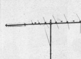
THESE TWO PHOTOS are examples of other shortcomings that were observed in local TV antenna installations. The set up in photo at left is good, but the broken lead-in wire waving in the breeze means that reception can't help but be bad. In the photo at right, both the VHF and UHF antenna are pointing in the same direction. This is a no-no because the signals for these two types of reception originate from
