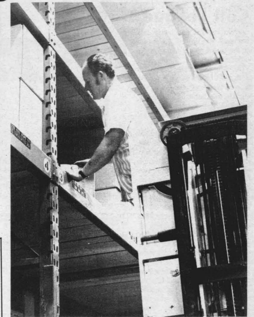
CLIFF MOSS, a stockman, pulls ordered items from a shelf while standing on the safety platform of a Crown lift. This machine is unique in that it allows the operator to remove items from 16 ft. shelves without assistance.
