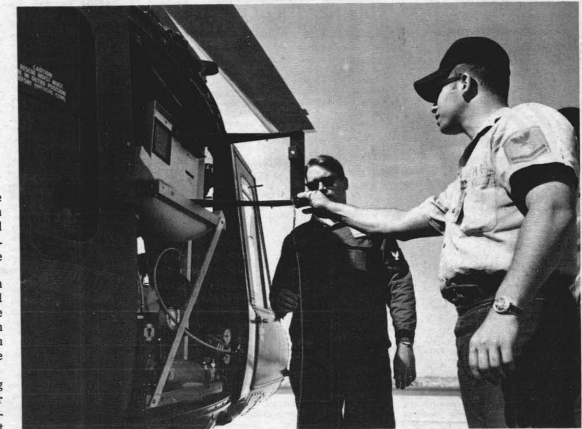
TEST PREPARATIONS MADE —Fire Control Technician 2nd Class Fred Morin (at right) is shown adjusting the scanning mirror before a laser equipped helicopter is sent aloft on a test run. Looking on is FTM2 Barry Ridenour. During night-time simulated air-sea search tests conducted here, packets of sea dye marker dropped into ponds have been readily visible to the helicopter crew—thanks to the laser beam scanner. —Photo by PH2 G. L. Taylor
