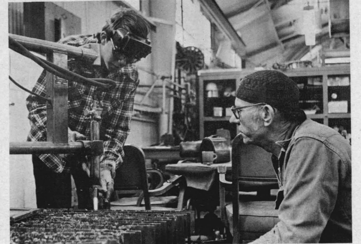
TIM MAHONEY, left, operates an automatic template burner under the supervision of Leo Carnahan, a welder in the Public Works Welding Shop.
