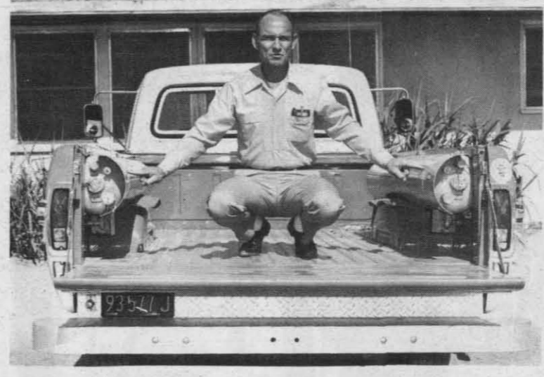
ANSWER TO CLEANER AIR—Eugene Copeland, an employee of the Refrigeration and Air Conditioning Shop, Public Works Department, points to the twin 23 3/4 gal. propane tanks mounted in the bed of his 1971 Ford pick-up truck. Copeland has mounted the fuel tanks in this manner so that he might also carry a camper shell. The NWC employee has been running his vehicles on propane since 1957.
