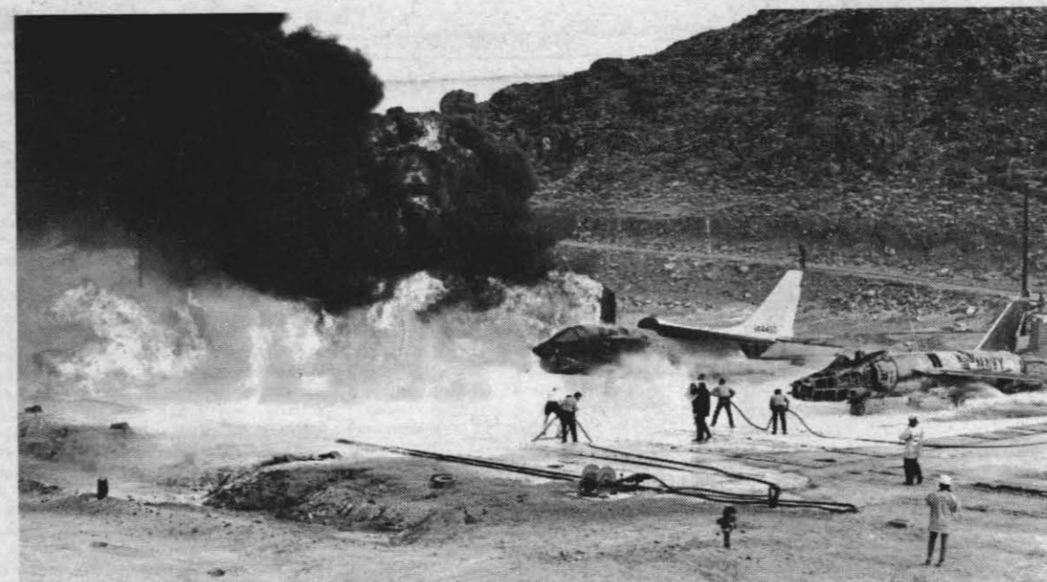
FIRE FIGHTING TESTS HELD—One of the current series of fire fighting tests being run by the Naval Weapons Center at the Mini-Deck Facility is shown above. The tests are being conducted in order to learn more about fire fighting agents and the techniques involved in the suppression of fires on aircraft carrier flight decks. Firemen seen in the foreground are members of the NWC Fire Department, who are assisting Code 572 in the tests.
