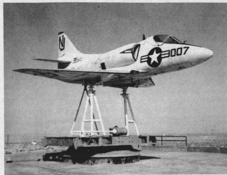
READY FOR TEST —An A-4 Skyhawk is shown on a tie-down stand that was fabricated from a 5-in. gun mount which was redesigned to support a full-scale test aircraft. Shortly after this photo was taken, the aircraft was subjected to continuous bursts of armor-piercing incendiary rounds that were fired into the plane's fuel tank below the surface of the fuel.
