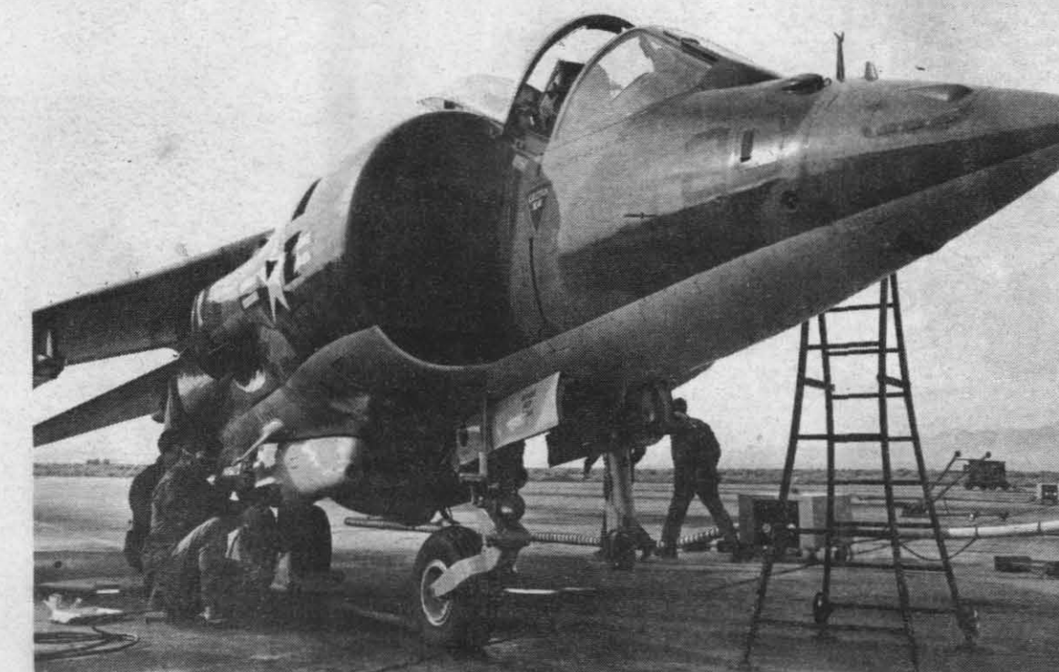
LOAD 30 MM ADEN GUNS — Personnel re-load the British-developed 30mm Aden guns on one of the Harriers. The Marines adopted the gun because it gives a high probability of first-burst hits when firing against ground targets. Marine pilots who have fired the gun like its low level of vibration and low rate of stoppages.
