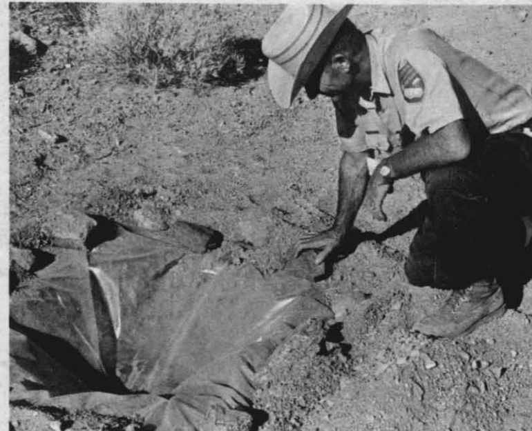
A SOLAR STILL is checked for moisture by the game wardens. The above photo was taken at 7:30 a.m. and the bottom photo shows two wardens checking at 4:30 p.m. In some places, the stills filled overnight with water enough to keep a person alive in the desert's heat.
