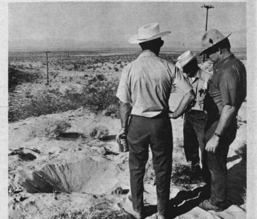
NOT ALL SOLAR STILLS work. Here DFG men survey a dry hole. It was found that holes dug in deep sand generally do not produce water. Stills dug in shallow alkaline areas (where dry lakes were found) produced the best results.
