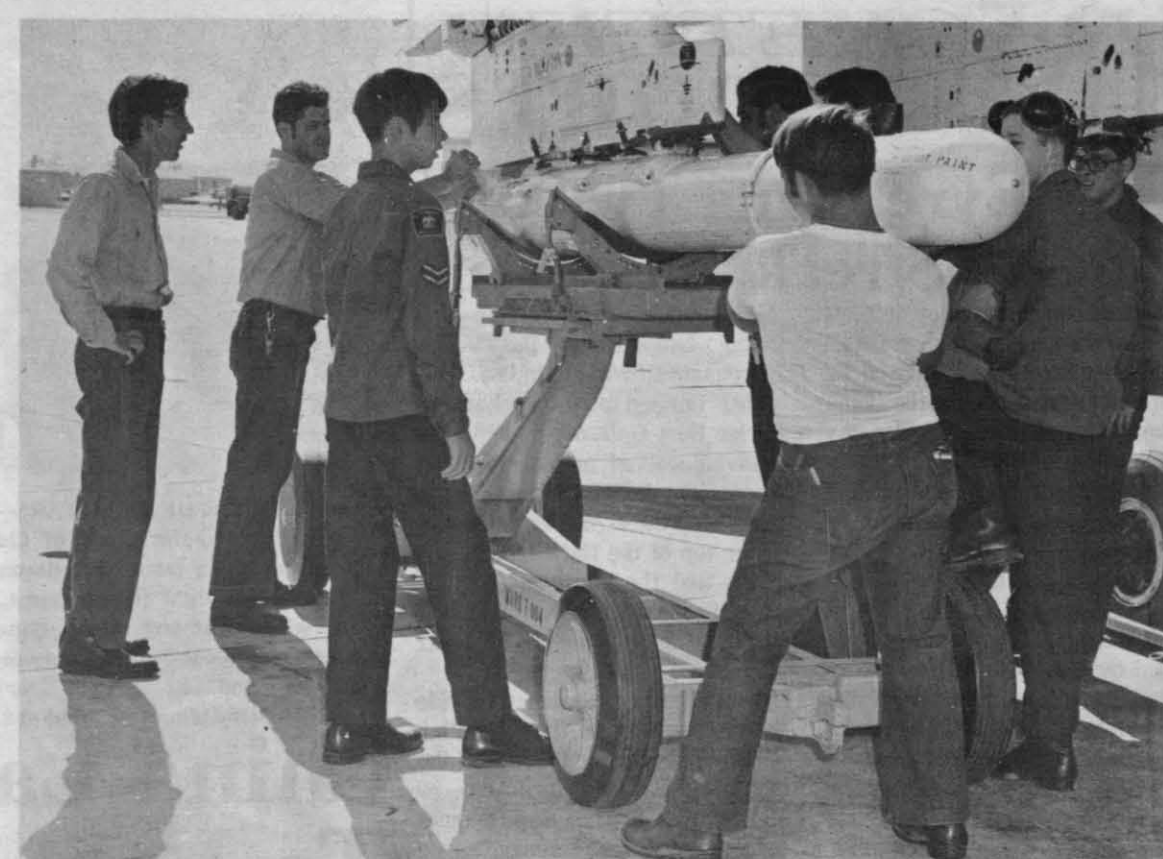
READYING AN A7E WITH A BEACON POD —Cadets and VX-5 ordnance crew members load an ECM Beacon Pod on an A-7E aircraft at VX-5. Cadets received instruction on mounting, handling and readying all types of ordnance during the 5-day seminar.
