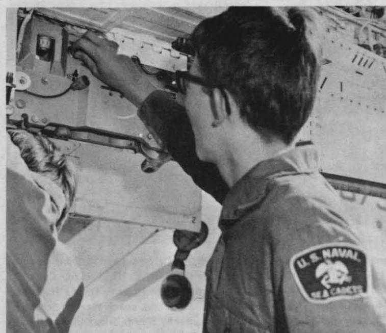
A CADET INSTALLS a safety pin in the BRU 10 Ejector Rack prior to mounting a ECM Beacon Pod on an A7E aircraft. This pin prevents the Pod from being fired accidentally while the aircraft is on the deck. Once the aircraft is readied for flight, the pin is removed.
